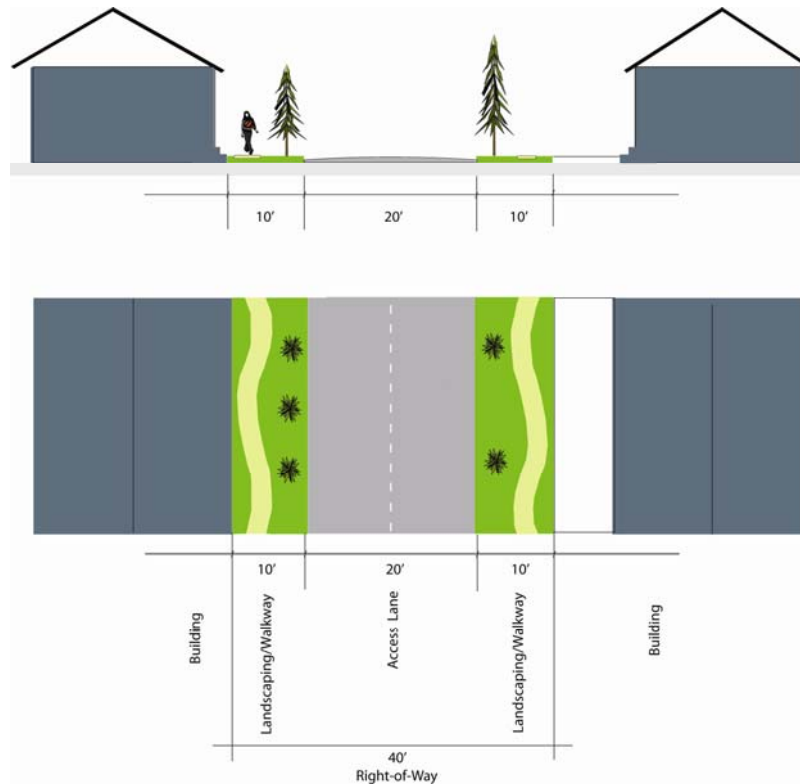
FIGURE 2-5 ACCESS LANE SECTION
