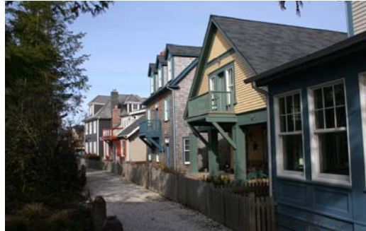
Figure 3B-6A: Do this Homes in Seabrook: Variation in scale and massing by utilizing varying roof planes
