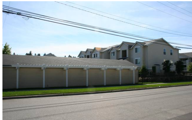
Figure 3D-10: Undesirable: Shared detached garage is oriented parallel to the street and presents blank wall to the sidewalk.
