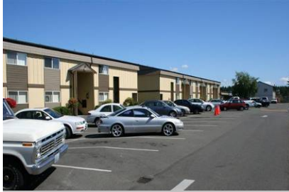
Figure 2-4 Large, impervious surfaces eliminate vegetation and prevent water from infiltrating into the ground
