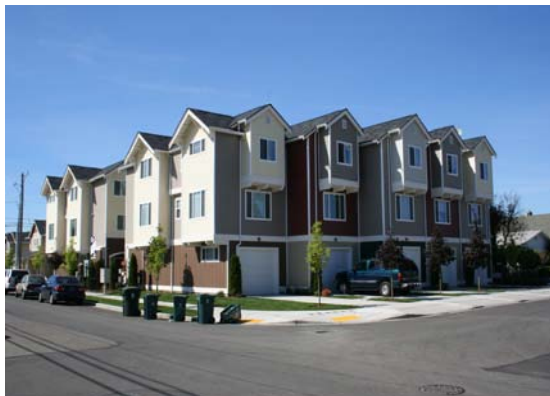
Figure 3D-22A: Undesirable: Parking is the dominant feature. Building frontage has a continuous driveway apron with no curbside parking.
