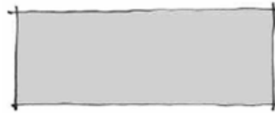
Figure 3B-5B: Don't do this -- Long unbroken walls appear massive
